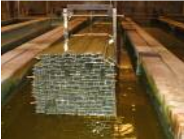
Replacing the hexa-valent chromium by chromium free substance in the powder coating line
